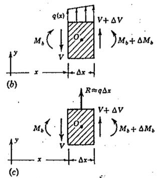
$$\Sigma F_{y} = V + \Delta V + q \Delta x - V = 0$$
